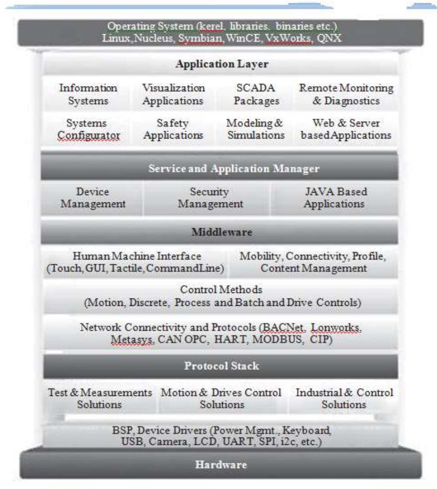
Figure 3.15 Middleware-based SCADA systems
