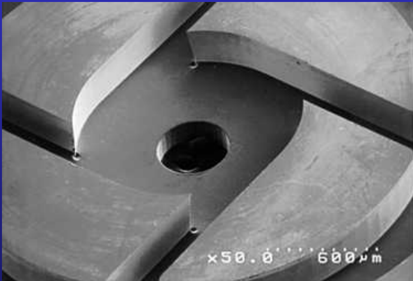
Swirl chamber and exit orifice of a fuel atomizer
