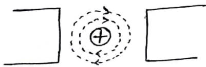
(b) Flux Produced by current carrying conductor.
