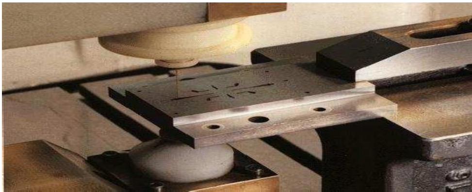
Figure: Wire erosion of an extrusion die
