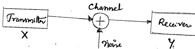
Let us consider transmitter  $X$  generating  $m$  symbols  $\{x_1, x_2, x_3, \dots, x_m\}$  with probabilities  $\{P(x_1), P(x_2), P(x_3), \dots, P(x_m)\}$
