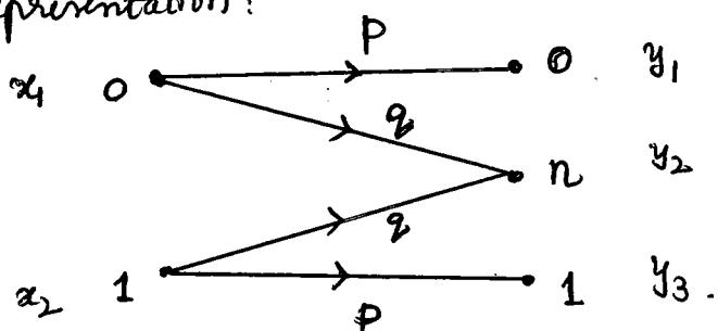
The channel matrix for binary erasure channel is
