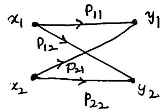
$$\Rightarrow \begin{bmatrix} P_{11} & P_{12} \\ P_{21} & P_{22} \end{bmatrix} \begin{bmatrix} Q_1 \\ Q_2 \end{bmatrix} = \begin{bmatrix} P_{11} \log P_{11} + P_{12} \log P_{12} \\ P_{21} \log P_{21} + P_{22} \log P_{22} \end{bmatrix}$$
