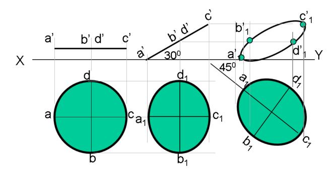
12. A thin rectangular plate of sides 60 mm x 30 mm has its shorter side in the VP and inclined at 30° to the HP. Project its top view if its front view is a square of 30 mm long sides.
