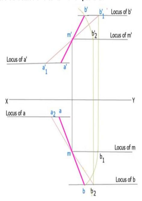
7. A line AB 60 mm long has its end B 20 mm above HP and 25 mm infront of VP. The end A is 50 mm above HP and 50 mm infront of VP. Draw its projections and find its inclinations with VP and HP.
