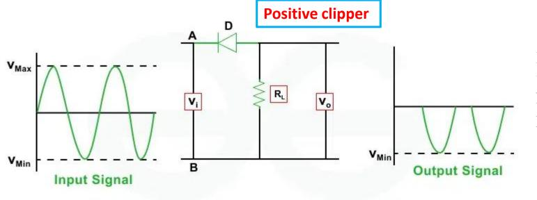
It removes the positive portion of an input signal's waveform, essentially "cutting off" the positive half-cycle while allowing the negative half-cycle to pass through. This is achieved by using a diode in series with the input signal.
