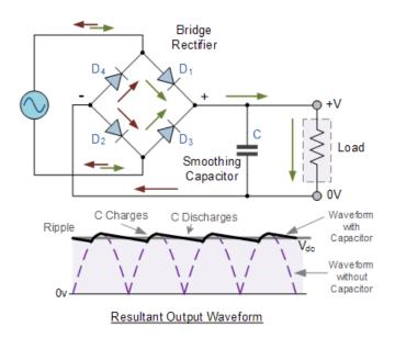
Another type of circuit that produces the same output waveform as the full wave rectifier circuit above, is that of the **Full Wave Bridge Rectifier**. This type of single phase rectifier uses four individual rectifying diodes connected in a closed loop "bridge" configuration to produce the desired output.
