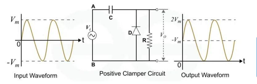
A positive clamper is a type of clamper circuit that shifts the entire waveform in the positive direction.
