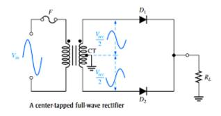
The full wave rectifier circuit consists of two *power* diodes connected to a single load resistance (R<sub>L</sub>) with each diode taking it in turn to supply current to the
