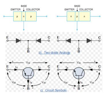
The transistor has three regions, namely; *emitter*, *base* and *collector*. The base is much thinner than the emitter while collector is wider than both as shown in figure. sake of convenience, it is customary to show emitter and collector to be of equal size.
