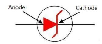
$\square$  As we keep increasing the reverse voltage it reaches a point where the reverse voltage equals the breakdown voltage. The breakdown voltage is represented as  $V_z$  and in this condition the current start flowing in the diode.
