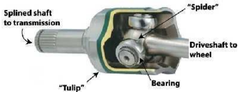
Cutaway view of Tripod "plunge" style CV joint
