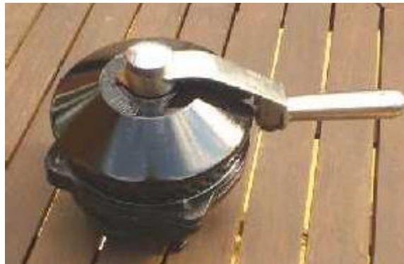
A driver's brake valve for a DMU. Photo: Traction ads.
