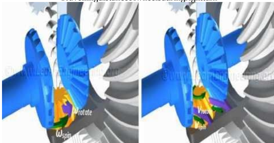
Direction of rotation of spider gear during right turn
