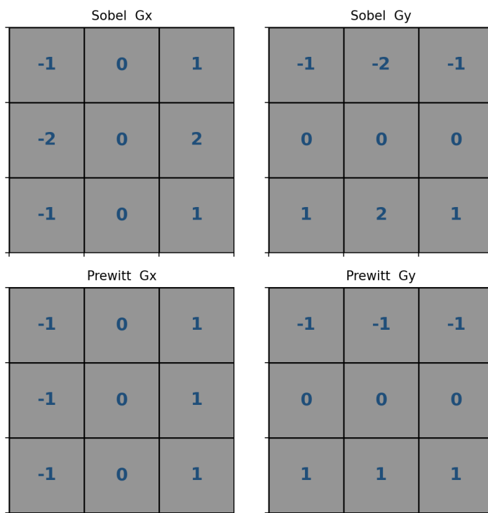
Fig. 2.7 — 3 \times 3 Sobel and Prewitt kernels for the horizontal ( G_x ) and vertical ( G_y ) gradient components. Sobel weights the central row/column by 2, giving mild additional smoothing.
